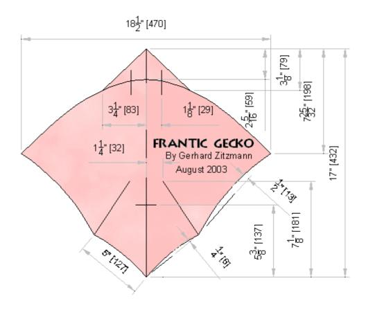
The frantic Gecko is a kite for light to middle wind conditions, the material I use is Orcon for the sail, the bow is 0.05 inch Carbon, the spine is made from Indonesian Bamboo and the battens are 0.03 Carbon. I saw a shape like this on a Custom made fighter from Paul Peters that was based on a fighter from Mike Coons, but I didn't find a plan like this in the web and so I make my own...
