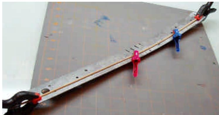
split has been 'reconstituted', clamp it and let the glue dry. Clamp the spine to a piece of metal such as an aluminum yardstick or ruler or a piece of construction metal. Pre-bend the metal to a shape that is similar to the bend of the spine in your best flying kite. The shape of the bend is something you'll want to experiment with to get the bend you like best.
