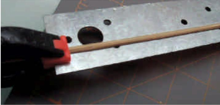
**A NOTE ABOUT CLAMPS:** One thing I noticed with clamps is that some have a strong enough spring to create a dent in the bamboo. The point where the dent is located is a weak point in the bamboo spine. Use clamps that will securely hold the two split parts together without denting the bamboo. That's why I use plastic clamps.
