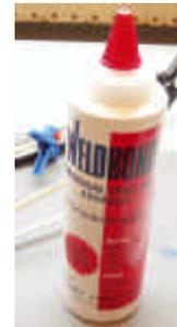
is a good tool for spreading the glue. I use glue by the name of 'WeldBond', it's waterproof white glue, but I think any waterproof wood glue or contact cement would work fine. I just happened to have some WeldBond so I used it. White glue remains slightly flexible after it dries, so the spine can be re-bent. If you use glue that is rigid when it dries the spine may not bend easily in the glued area after laminating. Choose the glue you think will work best for your desired result.
