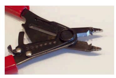
This is a wire cutter/stripper I bought for about \$9 at Home Depot. I removed the stop and filed off the teeth on the ends of the pliers so it would cut a 0.02" diameter rod in the 'V' cutter portion.
