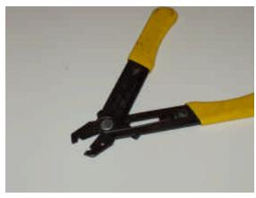
This is a less expensive wire cutter/stripper and works very well for cutting carbon fiber rods also. To make work for cutting carbon I removed the 'stop' so the 'V' cutting blade would cut small diameter rods.
