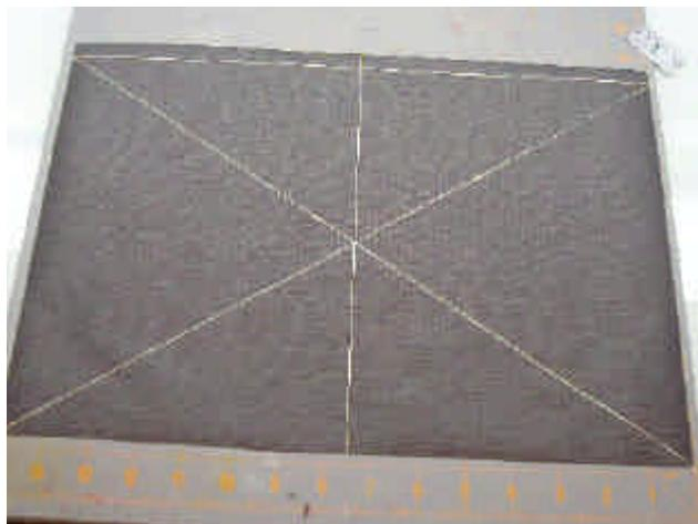
Measure a rectangle 10.5"/266.7mm x 15"/381mm on your skin material. This dimension includes a  $\frac{1}{2}"/12.7\text{mm}$  hem along the leading edge that will encase the leading edge spar.
