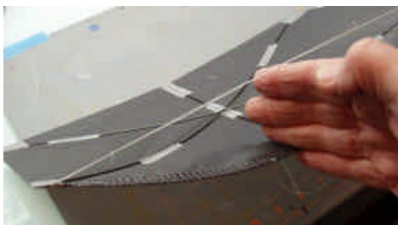
Before flying the buka, shorten the tension line which will create a bend or bow in the leading edge spar. The amount of bend you put into the leading edge spar will affect the way the kite flies. A very good average is to create enough of a bend so you can place 3 fingers stacked on top of each other between the leading edge spar and the tension line.
