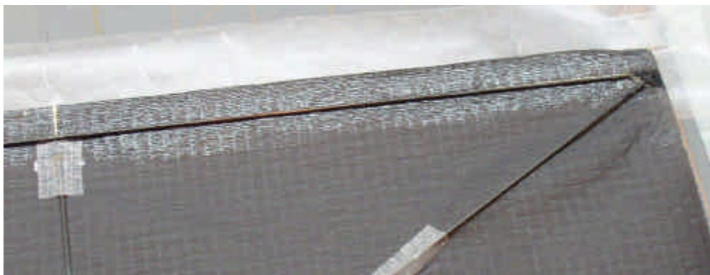
The leading edge hem is what secures the skin to the leading edge spar. The hem will be glued to the spar, using contact cement or a glue that bonds well to the skin material you are using.
