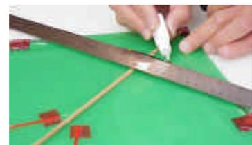
Also mark the location of the lower bridle connection at a point 6" toward the nose from the tail of the spine. Make a mark on either side of the spine at that point.
