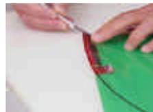
the carpet tape. Press the bow onto the carpet tape where it naturally touches it. Then, while holding down one side of the bow onto the kite skin, fold over the carpet taped wingtip hem tab around the bow and onto the kite skin. Burnish
