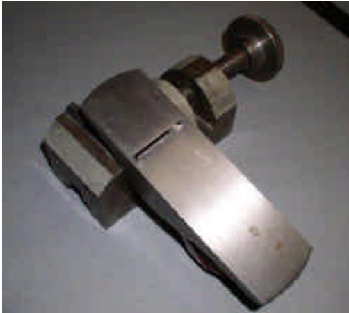
The plane clamped in a vise is what he uses for shaping his bamboo parts. He draws the bamboo across it as many times as necessary to shape the bamboo the way he wants it.
