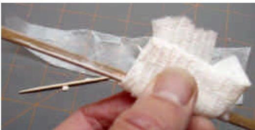
After applying the glue along the entire split surfaces, use a paper towel and bring the split parts together and wipe the excess glue from the spine. After the bamboo
