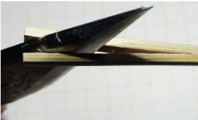
Cut the bamboo spine to the length specified by the kite plan you're using. Draw a straight line between the wingtips of the kite template or the cut out kite skin; this line is what I call the wingtip line. Lay the spine on the template or cut out skin and make a mark on the spine where the wingtip line intersects it.
